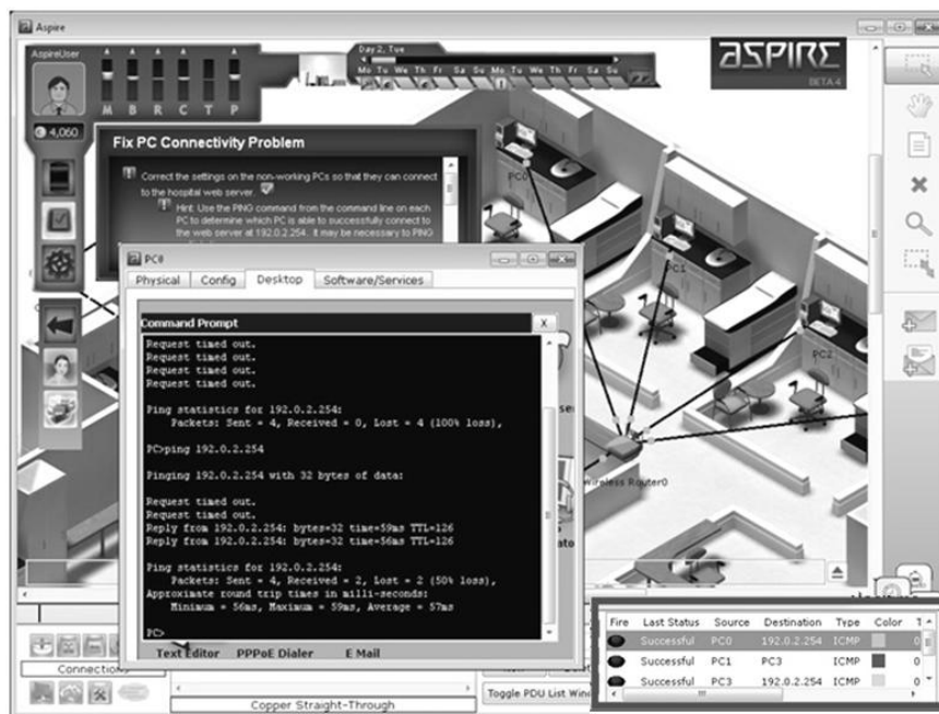
Figure 2. Screenshot of players using ping command and protocol data units for testing.
